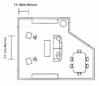
In an asymmetrical room, it is generally best to place the speakers facing the asymmetry. Try to keep the walls closest to the speakers at a similar distance.
